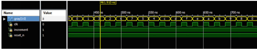
Fig. 18.11 Simulation result of 4-bit gray counter
