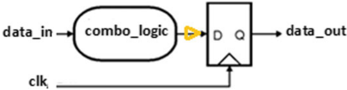
Fig. 15.16 Logic to fix the hold violation by using data buffers
